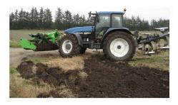
The high weight of the packer provides good packing and makes it easier to handle the plow.
