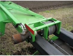
The packerunit consist of a frame with 2 rollers, either a tuberoller and/or cast iron rings. The unit has free movement, which limits the influences on the steering of the tractor.
