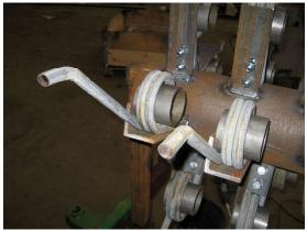
Very strong spring tines rotates with 180 n/min ( powered by tractor PTO ), grabs soil and plantmaterial and throws everything backwards in the air. The rotor works in 5 to 7 cm. depth.
